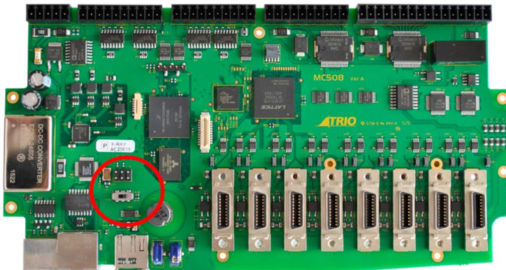
Temporarily replace the front of the MC508 back on to the chassis. Do not replace the screws.
